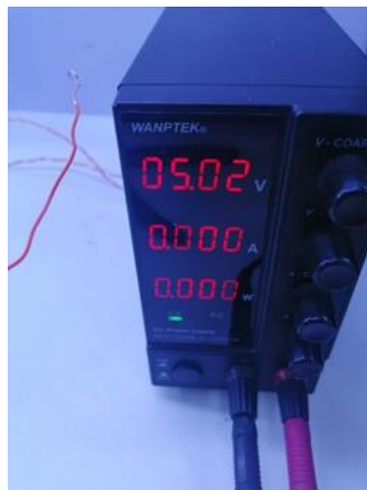
Figure 5.6: Power supply connected to pin 4 and 3.
