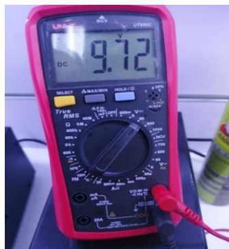
Figure 5.7: Analog output module multimeter test.
